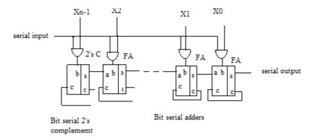
Figure 1: Serial by Parallel Booth Multiplier
